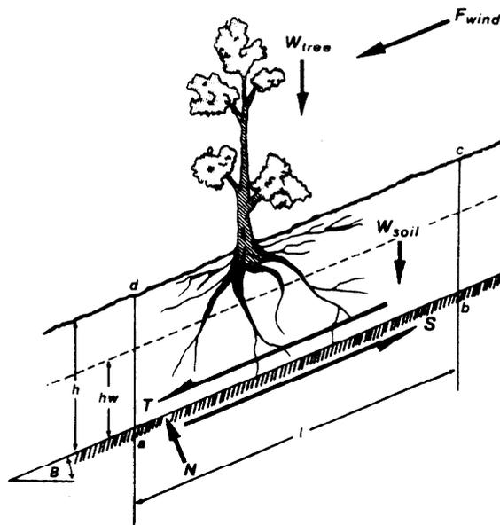
Figure 6. Part of a forested infinite slope showing forces operating on a sliding soil mass.
