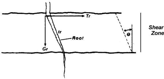
Figure 1. A well-anchored root stressed in tension where it crosses a soil shear zone.
