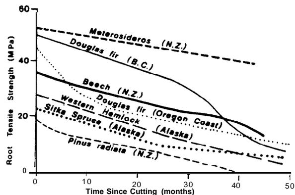
Figure 4. Curves of mean tensile strength vs time elapsed since tree felling for small roots of various conifer and hardwood trees,
