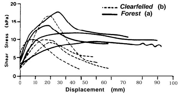
Figure 2. Shear stress displacement curves for field shear tests: (a) under intact beech forests, (b) on a slope clearfelled 36 months before testing.
