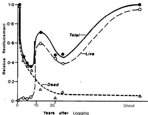
Figure 5. Relative reinforcement of soils by live roots generally increased while that by dead roots rapidly decreased with time after clearfelling. The total reinforcement by live and dead roots dropped to a low point about 7 years after logging (after Ziemer, 1981).
