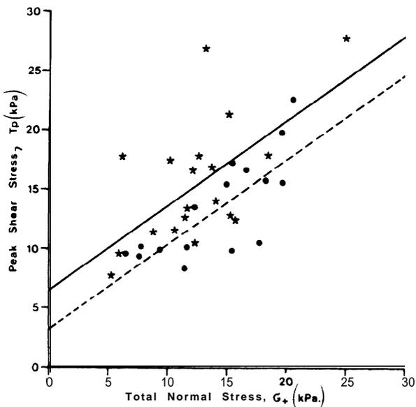
Figure 3. Fitted curves of peak shear stress vs total normal stress for field shear tests in the soil root zone; (a) beech forest (\*—), (b) clearfelled (• - - - -).
